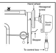
Mounting the Synchronizer onto the flange of hand wheel and match the stop groove of the synchronizer with the stopper of the machine head then tighten and secure 2 hexagonal screws of the synchronizer rotor, then connect the synchronizer cable to the control box.
