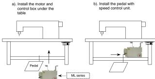
Note: ML series is designed for the H. S. mini motor, don't use with other brand of motor.(direct-drive motor is pre-installed on the machine head, if reinstall or disassembly is necessary, please refer to the sewing machine user manual.)
